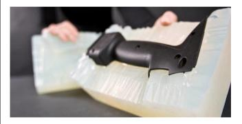
Max Dimensions: Dimensions are unlimited as components may be composed of several sub-parts. The build area of our largest machine is 700 x 900 x 750 mm
